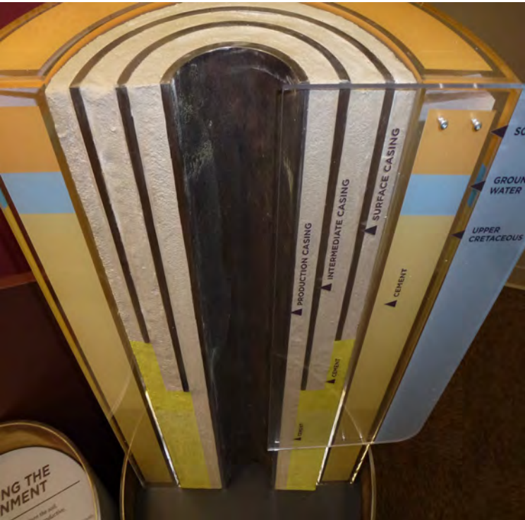
A cross-section of protective steel well casing cemented into a wellbore - on display in the Commission's Dawson Creek Resource Centre.
