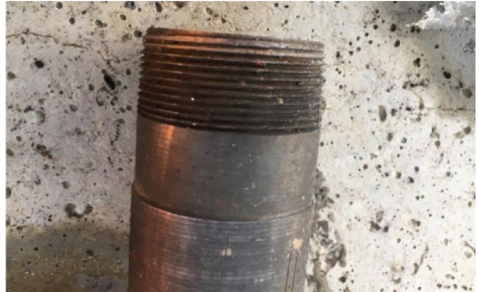
Figure 4: Bull plug recovered from base of the 'O' well showing damage on first two threads.
