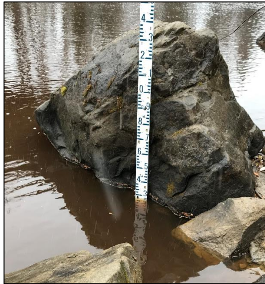
Figure 5. Staff gauge installed in stream and protected from ice and debris by rocks (photo credit – Suzan Lapp).
