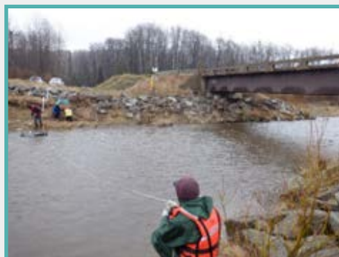
High flow discharge measurement on Hulcross Creek.
