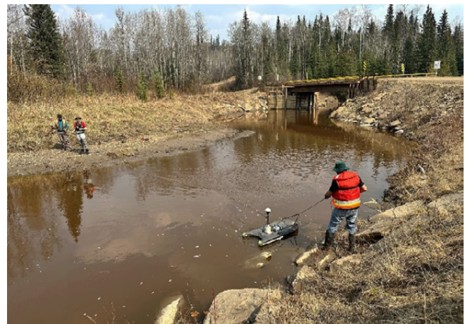
Environmental Stewardship team members measuring flow of Aitken Creek with a member of Blueberry River First Nations.
